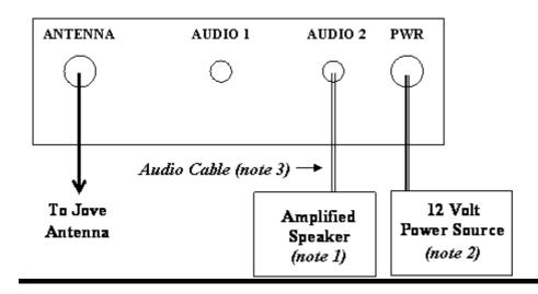
**Note 1** - The Radio Shack 277-1008 mini audio amplified speaker, which is powered by an internal 9V battery, is recommended. Alternatively you can use speakers that are part of a laptop computer (see advanced set-up). If you use amplified computer speakers powered by a separate power supply (the black cube type you plug into the wall) be aware that these supplies may cause hum and interference to the Jove receiver.
