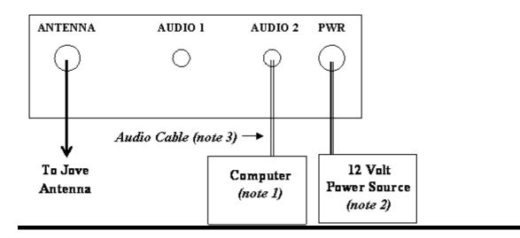
**Note 1** - The computer can be a notebook or desktop running Radio-SkyPipe software. Radio-SkyPipe has been tested to run on Windows machines using Win 98 or later and some Macintosh computers running Windows emulation software.
